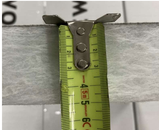
Ewona Acustica Luxury 50 mm HUSH fabric 52kg/m 3 , tile size 594 x 594 mm.
