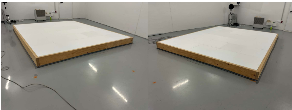
Figure A3.2. The specimen mounted on the wooden frame on the reverberation room.
