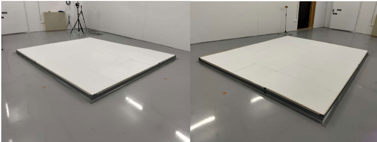
Figure A3.1. The specimen mounted on the floor of the reverberation room.
