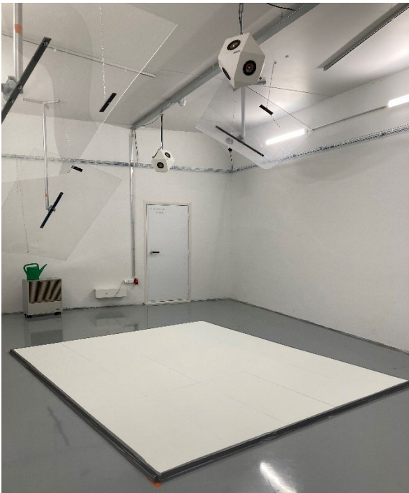
Type A mounting. Specimen on the floor.
